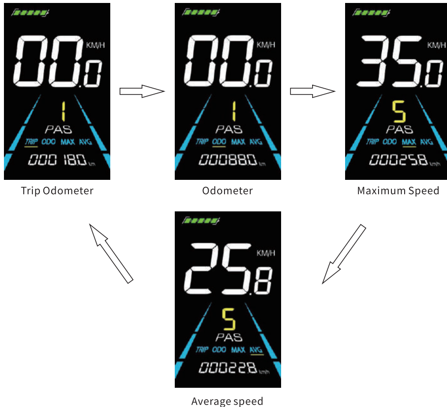
Figure 2-1 Display Interface Switching
