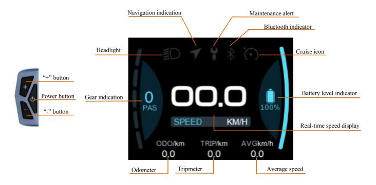
When the phone app connects to the Bluetooth of the meter, select the destination and start navigation after entering the navigation interface, the main interface displays the following changes:
