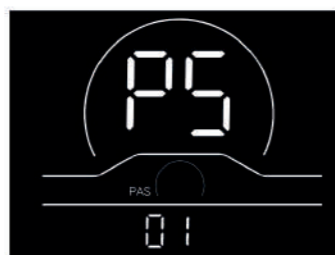
Fig. 4-5 Speed Sensor Setting Interface
