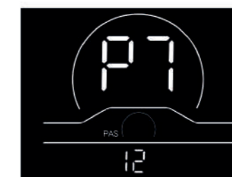
Fig. 4-7 Assistance Sensor Setting Interface
