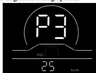
Fig. 4-3 Speed Limit Setting Interface
