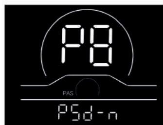
Fig. 4-8 Power-on Password Setting Interface
