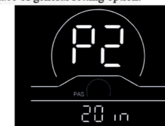
Fig. 4-2 Wheel Diameter Setting Interface
