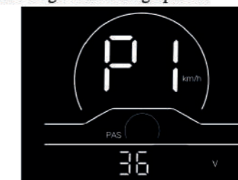
Fig. 4-1 Rated Voltage Setting Interface
