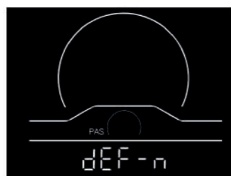
Fig. 3-1 Factory Reset Interface
