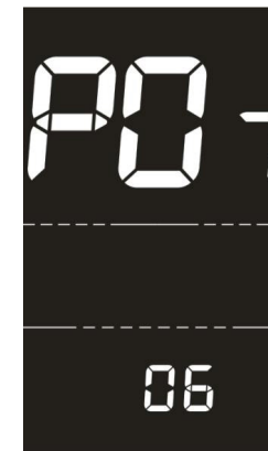
Setting interface of magnetic steel number of speed measuring sensor
