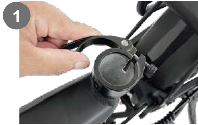
1. Open the quick release lever by swinging the lever open and outward fully.
