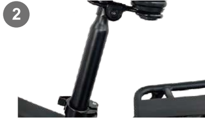
2. Move the seat up and down by sliding the seat post in or out of the seat tube. DO NOT raise the seat post beyond the minimum insertion marking etched into the seat post tube.
